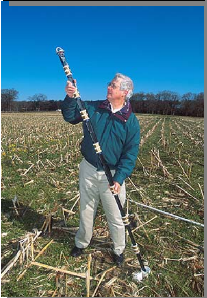
OPE3 scientist inspects Sentek EnviroSCAN soil probe.
